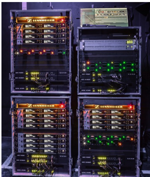
Autograph supplied 32 channels of Sennheiser's Digital 6000-series to Curve, ready built into one 16-way and two 8-way racks, all complete with custom-made panel work for AES and analogue outputs plus data and antennae patching, plus internal power distribution on each
